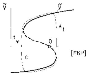
Fig. 4. Limit cycle  $C$  around an unstable stationary point  $O$ . Arrows indicate direction of the oscillatory motion in the futile cycle (15).
