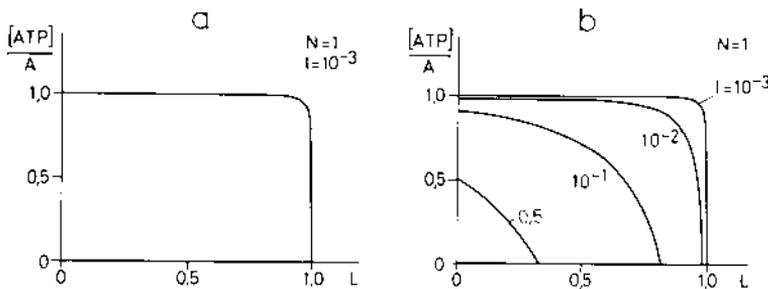
Fig. 1 (a). The stabilization of ATP concentration by CEM (3) within a wide range of relative load activity  $0 \leq L < L^*$ . (b) Disappearance of ATP-stabilization with increase of relative leakage activity,  $l$ .
