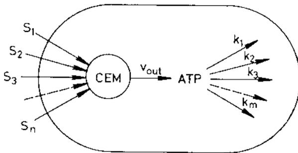
where  $S_1, S_2, \dots, S_n$  are initial substrates of CEM;  $k_1, k_2, \dots, k_m$  are rate constants of  $m$  different ATP-consuming processes;  $v_{out}$  is the output velocity of CEM.
